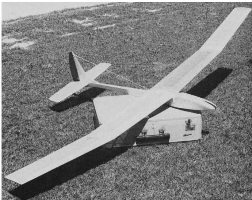
Don McGovern's "Wild Blue" soarer will disassemble and fit into the suitcase for easy transportation. Zaic's "Scout" (opposite) is a stubby contrast to the conventional long-wingers.
